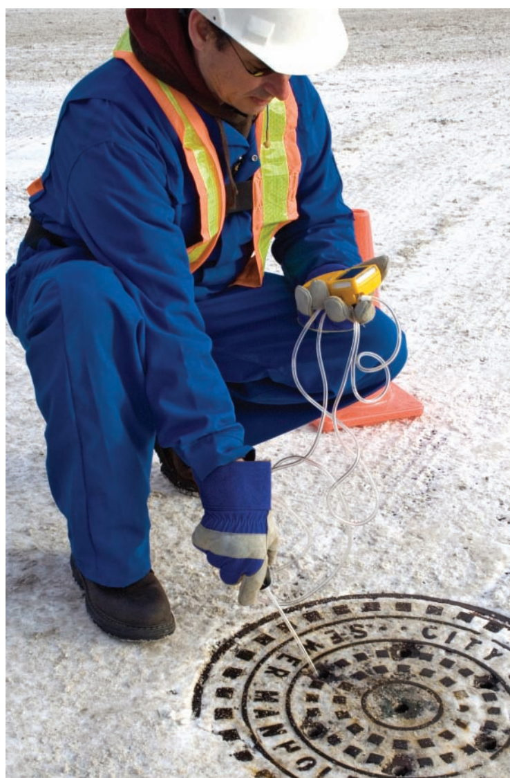
Testing the atmosphere with an appropriate, properly functioning, safety gas detector is the only way to determine whether it is safe to enter.
