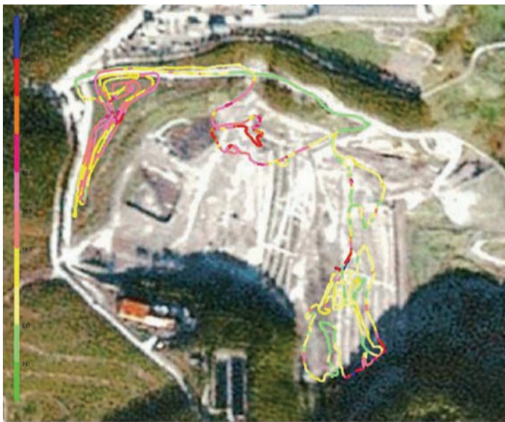
Figure 4: GasFinderVM survey of near ground CH 4 concentrations at a landfill in Spain
