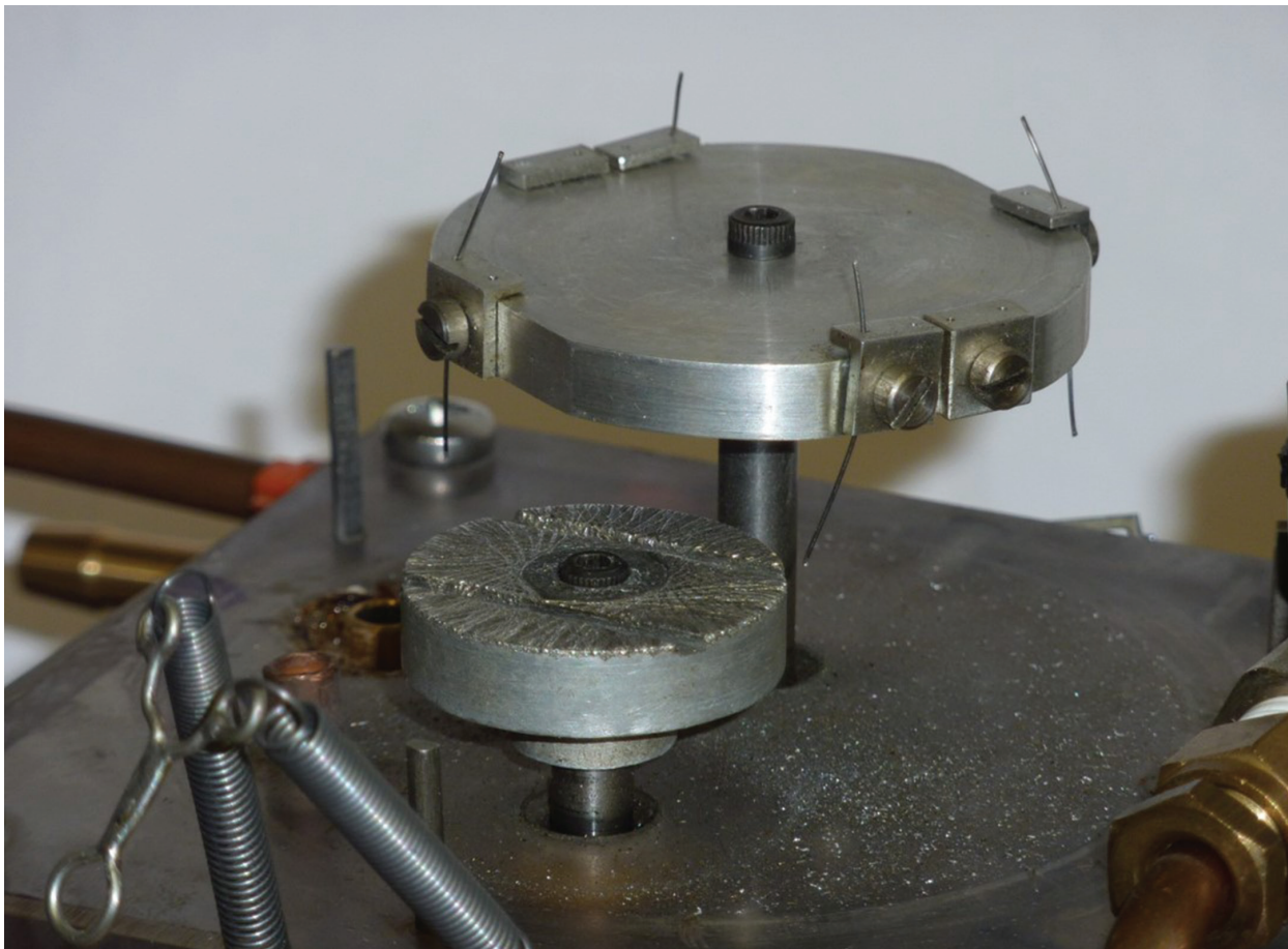
IEC TC31 is concerned with the health issues of continuing to use a cadmium disk as the main test resource for intrinsic safety
