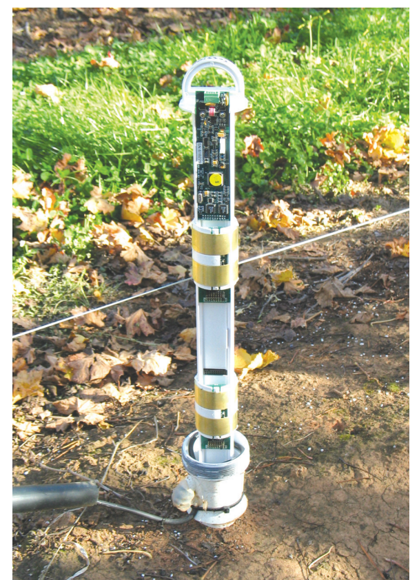
Sentek EnviroSMART capacitance probe, showing annular electrodes and top of access tube. Picture courtesy of Campbell Scientific Ltd
