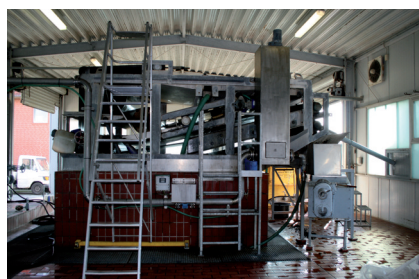
Fig. 8: Belt filter press for sludge
