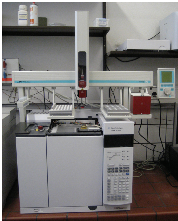
Image 3: A Combipal auto sampler with HS module on a Agilent GC
