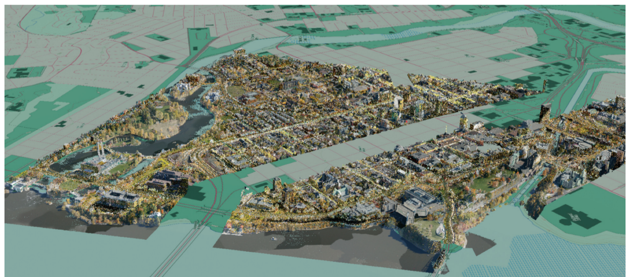
Figure 4: A screen shot of a colour point cloud consisting of over 1 billion individual points from a LIDAR survey of downtown Ottawa, Canada which is overlaid on a map streamed via a web map services provider. Trees, people, and cars are visible at close range. LIDAR data provided by dayta Ohio.
