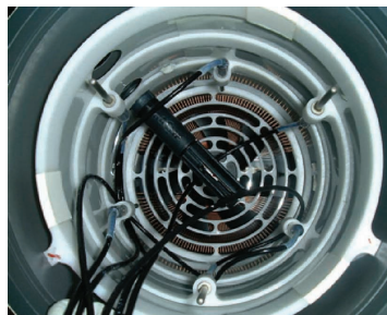
Figure 7: Six PRT array used to measure 5 temperature gradients
