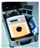
Designed and manufactured by **Hidex** (Finland), the Triathler<sup>™</sup> multilabel tester allows sensitive on-the-spot measurements of alpha, beta and gamma radiation as well as luminescence.
