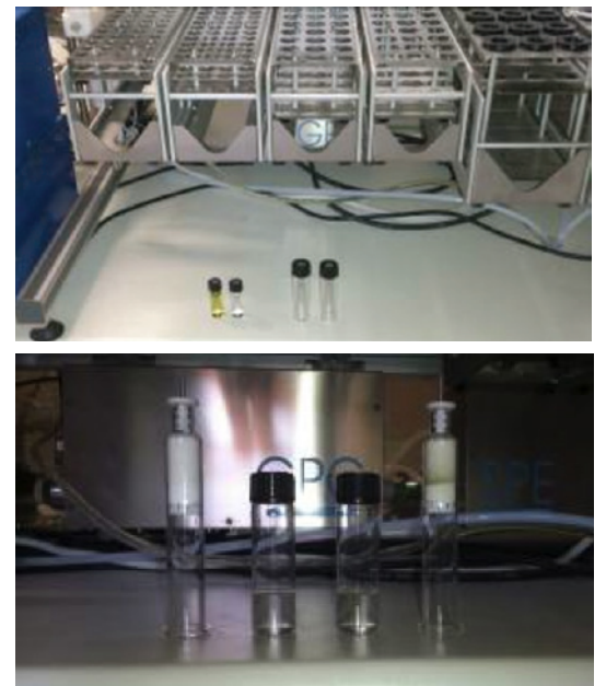
The sample extract is placed into the FREESTYLE™, then loaded fully automatically onto the pre-packed Elufix™ column and eluted in the evaporation unit. Here, the volume is reduced to an end volume as defined in the method and then transferred into a sample vial.
