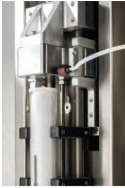
Figure 2 The device, which emerged from the collaboration, is characterised by a particularly simple mode of operation. Preparatory work includes only the connection of collection vessels to the output lines and clipping the ready-to-use columns into the holder – the other system's standard screw connections are omitted, the locking is done by the system.
