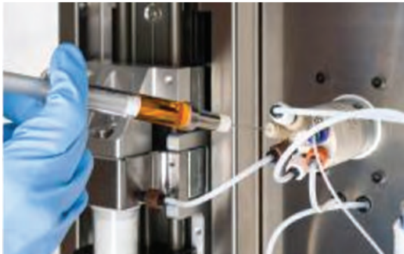
Figure 3 Injection into the sample loop is the only manual step of the entire preparation process, everything else runs fully automatically after you start the device.
