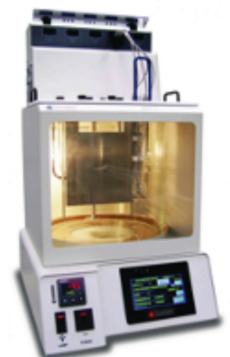
Figure 3. KV5000 Koehler Kinematic Viscosity Bath with Optical Flow Detection System [14]
