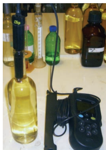
Figs. 3 and 4: Oxygen measurement in a bottle with HQD and LDO sensor
