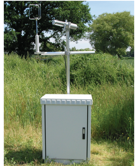
Typical Eddy Correlation site. Picture courtesy of ADC BioScientific.
