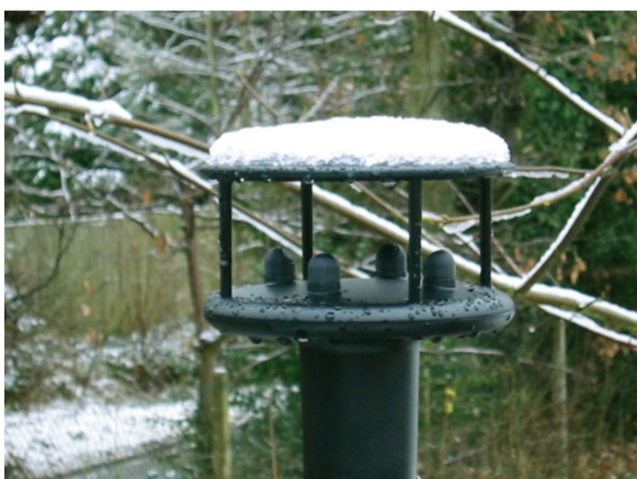
Two axis ultrasonic anemometer. Picture courtesy of Gill Instruments.
