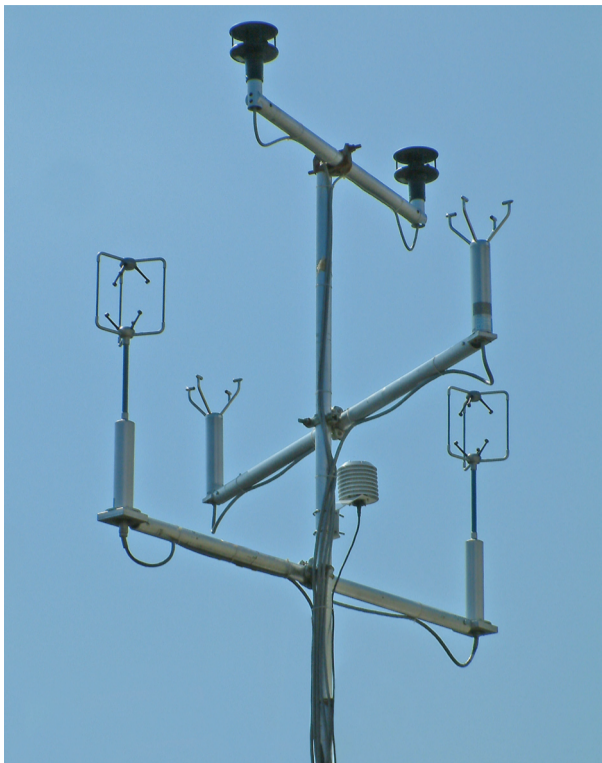
Typical array of two axis and three axis anemometers. Picture courtesy of Gill Instruments.
