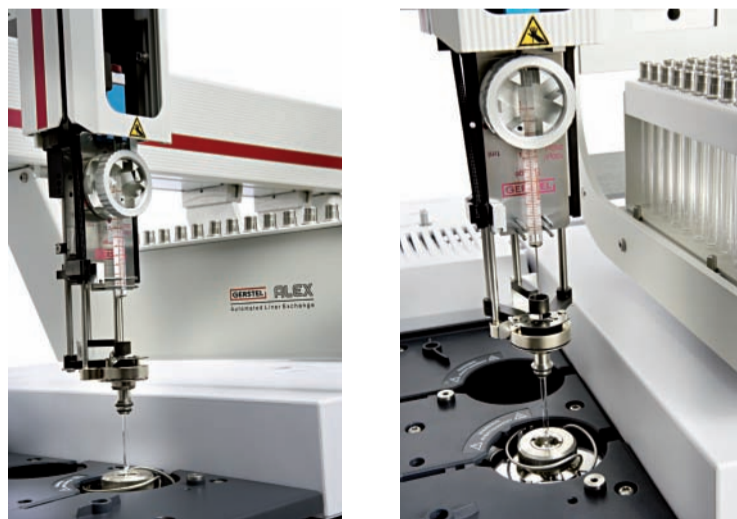
Figure 1: Automated Liner Exchange (ALEX) installed on an Agilent 7890 GC equipped with a CIS 4 programmed temperature vaporisation (PTV) type inlet. Detailed view of the ALEX System.
