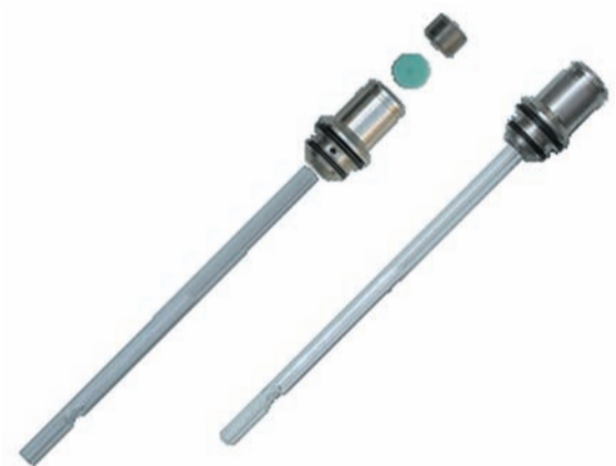
Figure 2 Left: Exploded view of transport adapter for automated liner exchange with liner, adapter, 3 x 5mm septum and septum screw; a hole for carrier gas entry can be seen between the o-rings of the transport adapter. Right: Assembled transport adapter with liner
