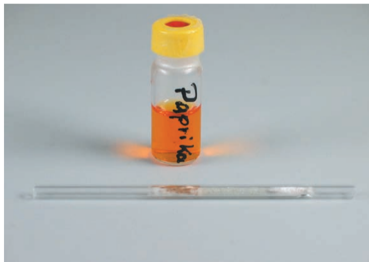
Figure 5: 2 mL Vial containing a QuEChERS method bell pepper extract and a liner packed with glass wool in which 5 \mu L of this extract has been injected.
