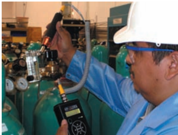
Hydrogen leak detection
