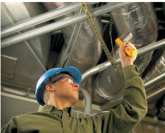
Fig 1: Non-contact infrared thermometers offer a fast, safe and accurate method of measuring surface temperature.
