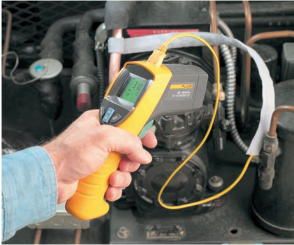
Fig. 4: The Fluke 561 multipurpose thermometer combines a contact and non-contact (infrared) thermometer into one portable tool.
