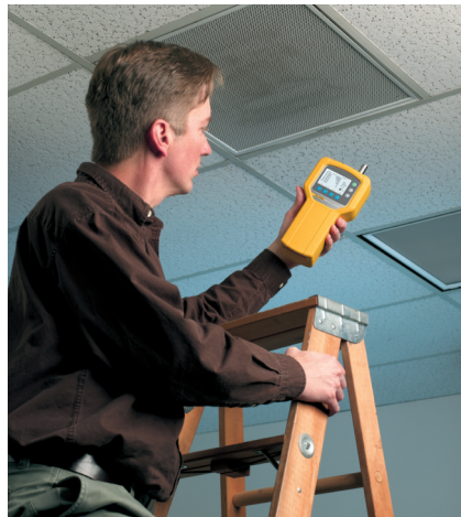
Airborne particles come in a number of shapes and sizes, which can be accurately identified and quantified with a particle counter, such as the Fluke 983 shown here.
