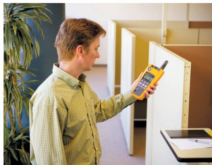
Reading CO 2 levels in an office space with the portable Fluke 975 AirMeter tells you whether ventilation is sufficient. This tool also measures temperature, humidity, air velocity, and carbon monoxide levels.
