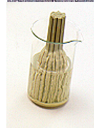
Direct Well with bentonite collar slipped on riser tubing
