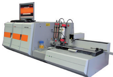
Figure 2: multi EA ® 4000 with TIC automatic module and solid sampler FPG48 for the automated determination of different carbon species in solid and selected liquid samples
