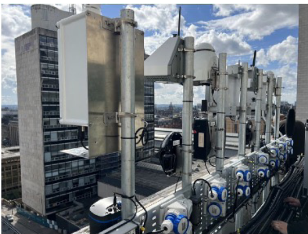
Figure 2: Phase 1 test site: rooftop base station in central Glasgow, with a large array of AQ sensor attached to it
