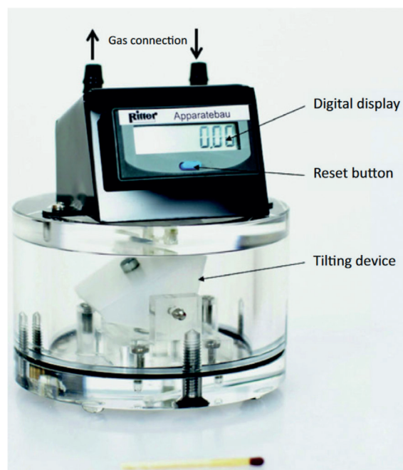
Fig. 4: MilliGascounter for detecting low gas flows according to Scherer
