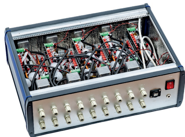
Fig. 3: Array of 9 INFRA.sens® gas measurement modules for measuring the CO 2 and CH 4 gas concentrations in the respective fermentation vessels with internal tubing (Viton®)
