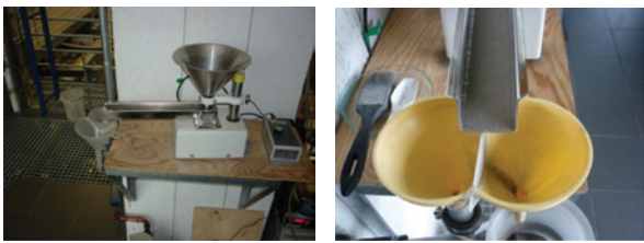
Fig 2. Vibration dust batcher for the dust train
