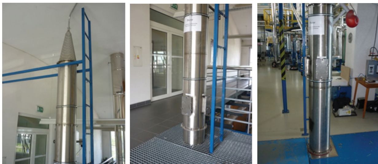
Fig 3. Diluting section on the left, measuring profile 1 (upper) in the middle, measuring profile 2 (lower) on the right
