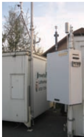
Figure 1: airpointer® compared to a traditional measuring station on the occasion of the Steyregg round robin test [1]
