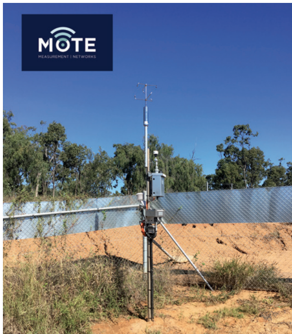
Mote CVM Dust Tower
