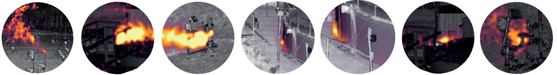
Plumes of gas characterised at QLM's recent trials at NGG's Bacton Terminal, METEC, and Severn Trent's Minworth Sewage Treatment Works, showing methane concentration as a "heat map" over the lidar background
