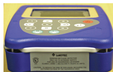
A GEM 2000 Plus Gas analyser with its USA UL Label
