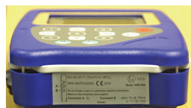
A GEM 2000 Plus Gas analyser with its European ATEX Label
