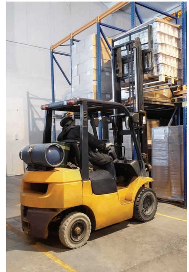
Image 4: Forklift Trucks are commonly used indoors in manufacturing and warehouse facilities, they can emit potentially dangerous levels of Carbon Monoxide
