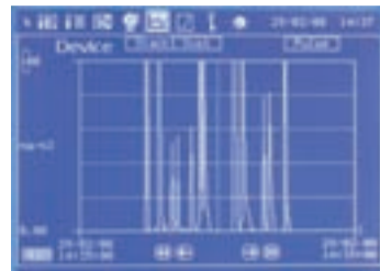
Dynamics of dust levels during filter cleaning and monitored to diagnose location of leaking bags
