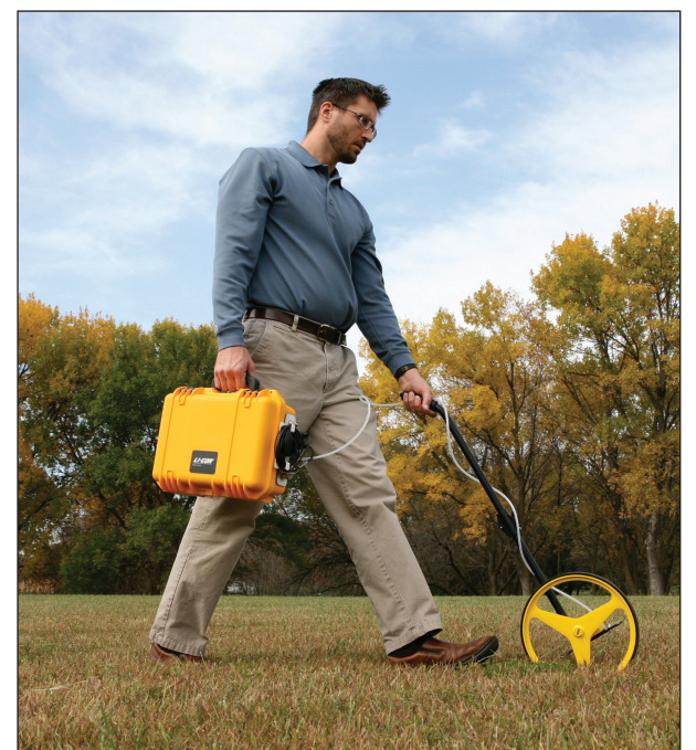
Measuring ground level CO 2 concentrations with the LI-8100A Automated Soil Gas Flux System.
