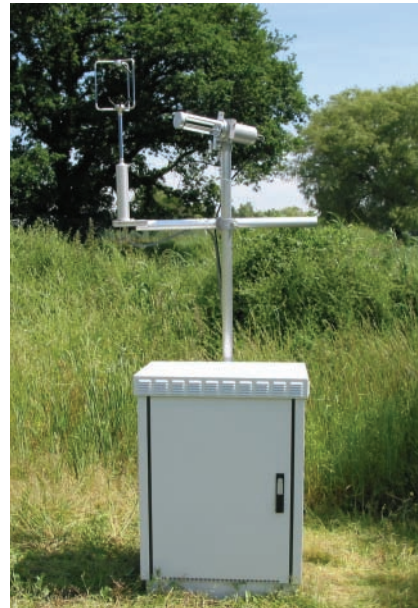
Typical Eddy Correlation site. Picture courtesy of ADC BioScientific.
