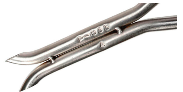
Figure 2 - S type pitot head
