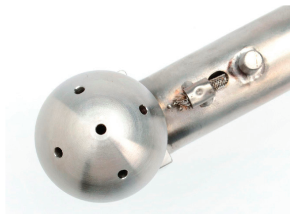
Figure 1 - 3D pitot head
