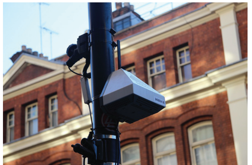
“One of 100 AQMesh pods installed during the Breathe London pilot
