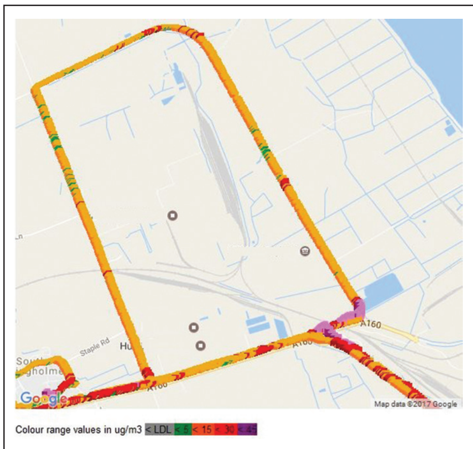
Figure 1: Benzene levels from Duvas gas test at areas surrounding Immingham chemical plants, Aug 2016
