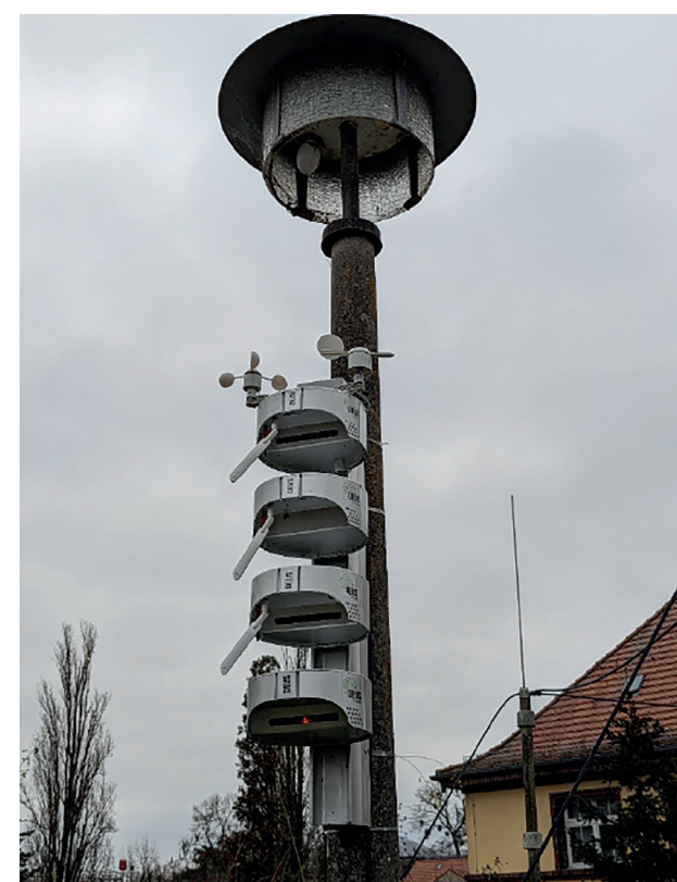
Figure 1: DEUS-Pollutrack measurement units (four modules, the first module from the top: measuring wind speed and direction as well as precipitation, the second: CH 4 , the third: CO 2 , NO 2 , and VOCs, and on the bottom: particulate matter (PM 1, 2.5, 10))
