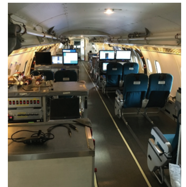
The inside of the plane has been stripped right back to allow more space for instrumentation
