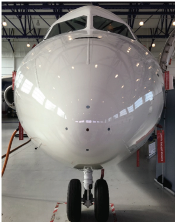
The FAAM CORE 5-hole turbulence probe, measuring incident airflow and 3D wind components
