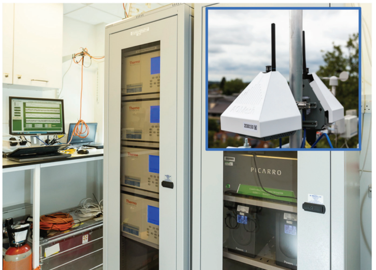
Figure 1. Traditional Air Quality Monitoring analysers and low cost air quality network node (top right corner, courtesy Environmental Instruments)
