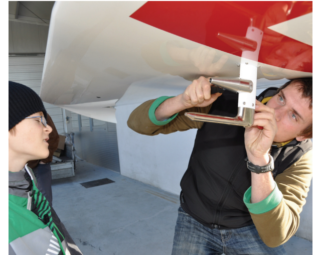
Fitting an aerosol inlet for an Aethalometer to measure Black Carbon
