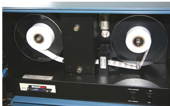
Aethalometers employ an optical method to only measure those fine particles which are black
