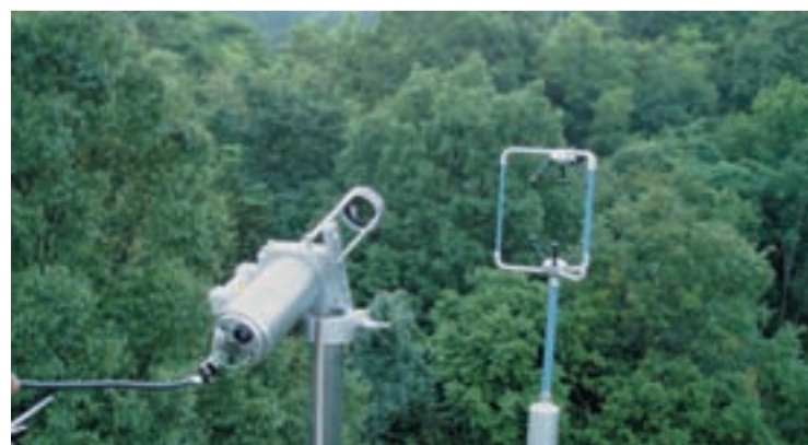
ADC OPEC system at CFERN field station Jianxi Province, China.
