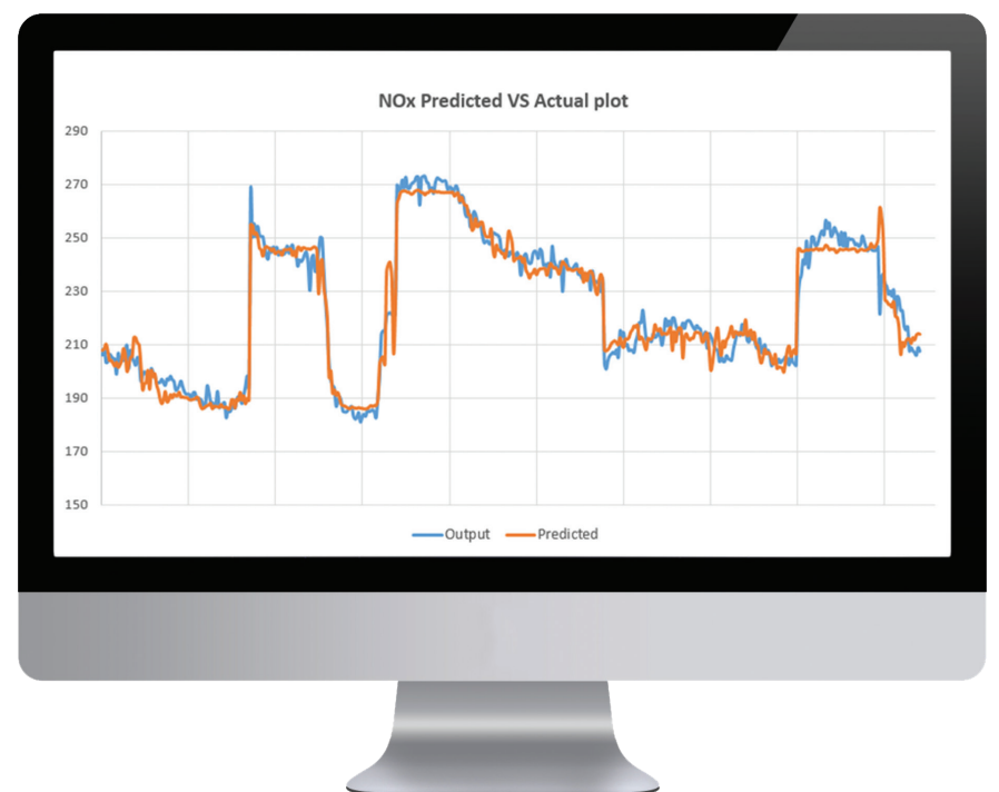
Predictive emission monitoring systems (PEMS) are increasingly being used for monitoring and recording air pollutant emissions.
